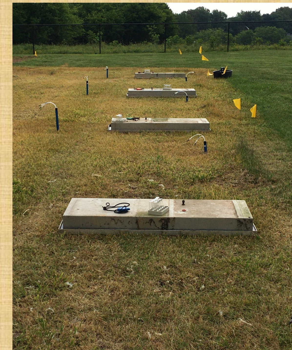
Gas flux chambers to quantify N 2 O emissions
