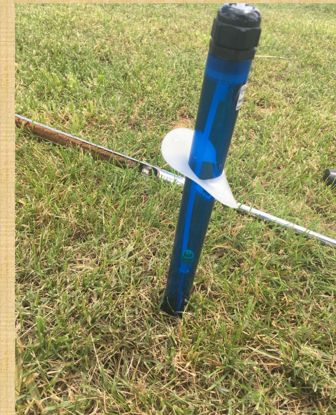
Lysimeters placed at 15 and 30 cm deep to collect NO 3 - leachate
