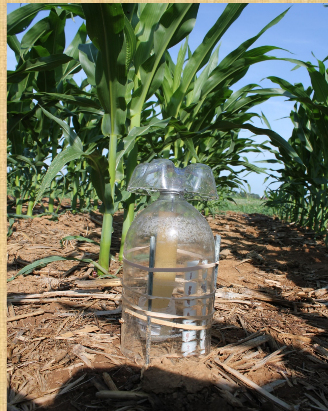
Semi Static Chambers to quantify NH 3 volatilization
